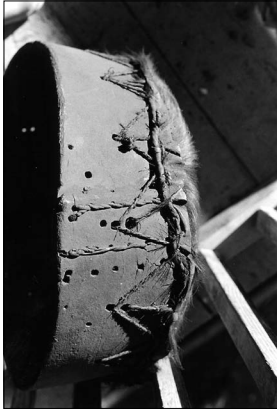
Fig. 7. Way of fastening membrane
