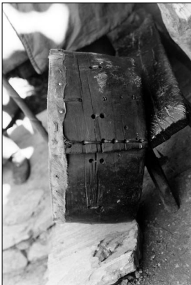
Fig. 9. Overlapping ends of drum frame clamped together
